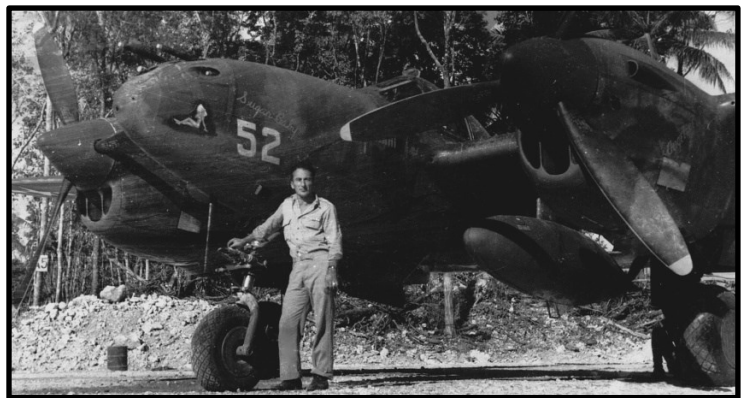
This photo shows the business end of the Lightning with four 50 caliber machine guns and a 20 mm cannon mounted in the nose. A 165 gallon drop tank is mounted under the wing.
